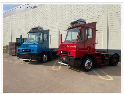
Bettaway recently purchased and put into service two new all-electric yard tractors, which move trailers to and from loading docks and yard staging areas.
