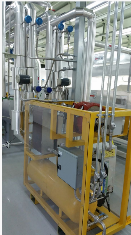
Infinity Turbine IT10 10 kW System Using Industrial Waste Heat
