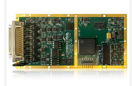
The HPx-450 card has a dual set of inputs, allowing 2 radars to be connected.
