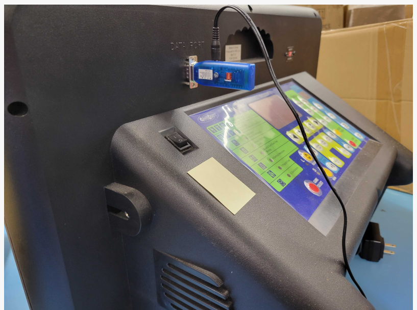
A GRIDBluFly adapter connected to the serial data port of a scoreboard display for remote access via Bluetooth.
