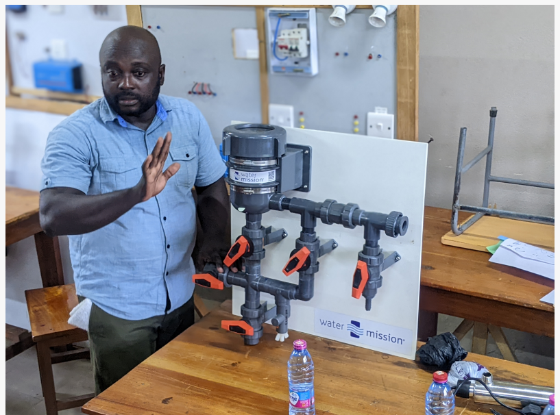
Mawuli Tsikata, Assistant Manager, Technical Services at Safe Water Network, explains to participants how a chlorinator works
