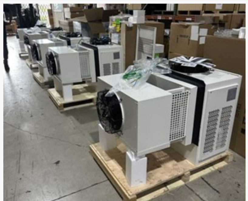
Single Phase Chillers and Freezers at USA Containers Workshop
