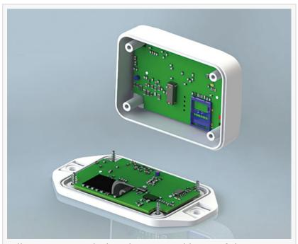
Pillars are provided in the top and base of the DATA-MOBIL-BOX enclosures for mounting the PCBs.
