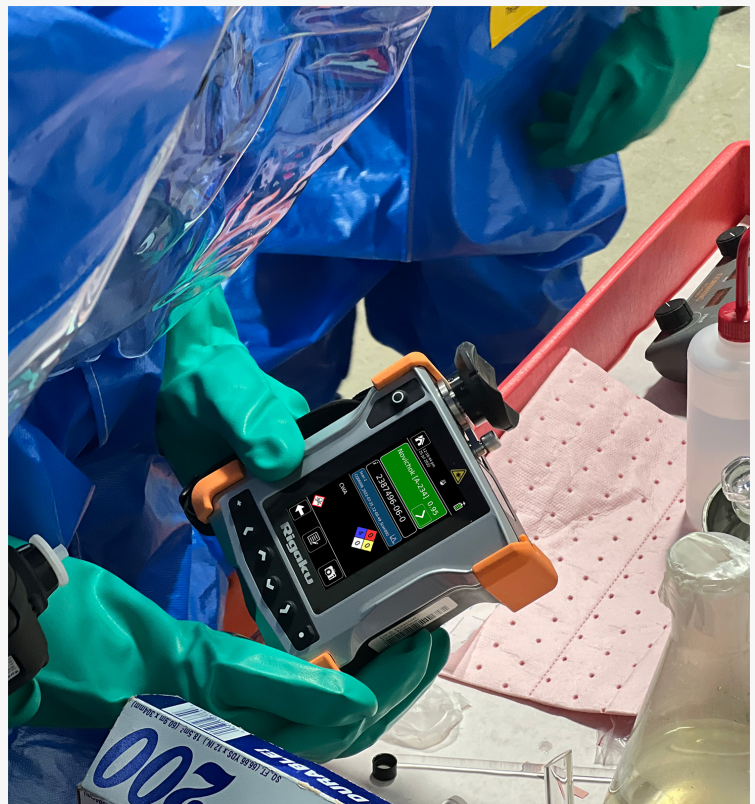
Rigaku CQL Max-ID handheld 1064 nm Raman analyzer identifying Novichok chemical weapon.
