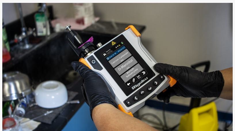
Rigaku CQL Max-ID handheld 1064 nm Raman analyzer identifying mixtures.
