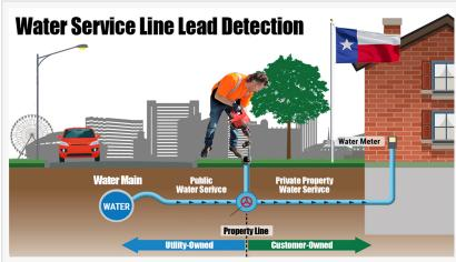
Instead of digging or excavating, the Electro Scan SWORDFISH is able to assess buried lead pipe on both the Utility-side and Customer-side of a meter or curb box.
