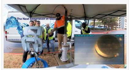
Electro Scan's TRIDENT combines CCTV and Electro Scan Electrical Resistance Testing to locate leaks, measure leakage flow rates in Gallons per Minute, and map internal pipe corrosion.
