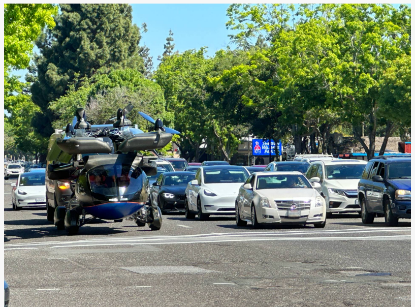
ASKA A5 drive & fly eVTOL road testing
