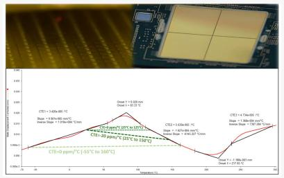
A new class of low dielectric constant (2.6-2.8) and loss Build-Up Film prepregs based on AIT's established modified cyanate ester film technology demonstrated here with CTE controlled close 8 ppm/°C with molecular stress absorption and high temperature d
