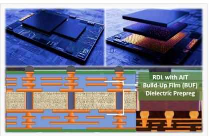
One of the critical properties of a successful Build-Up Film (BUF) dielectric prepreg adhesive is the ability to match the CTE of the core BT substrate (12 ppm/°C) and copper (18 ppm/°C) in minimizing the interfacial stresses while maintaining high melt-f
