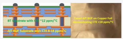
Copper pillar interconnections or gold-stud bumps is best with underfill CTE less than copper at 18ppm/°C. Chip-on-package such as BT or equivalent having CTE of 12 ppm/°C is best matched with Build-Up Film layer each with CTE as close to 12 ppm/°C as pos
