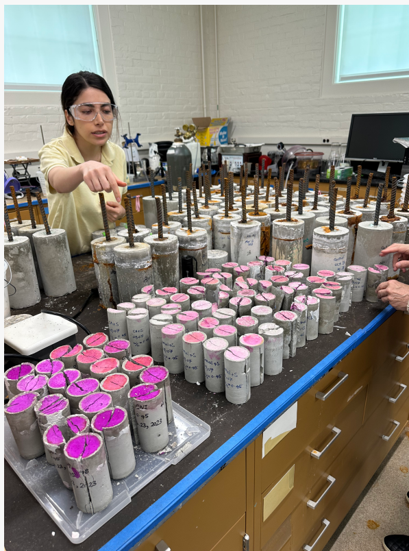
Sara describing our Accelerated Corrosion Test with many ECI supplemented samples.
