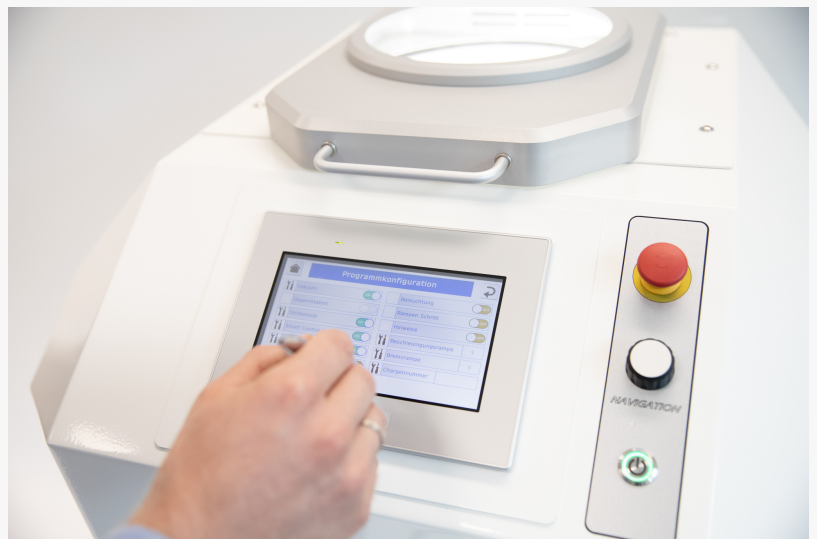
Mixing new formulations for composites with the Hauschild SpeedMixer® with sensor integration and automatic pot cooling system
