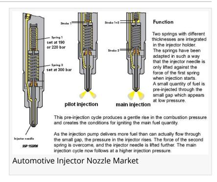
fuel by making a fine mist of the fuel, so that there would be complete and effective combustion of the fuel for driving with better efficiency.
