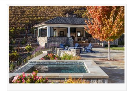
boundary wall that holds the water appears not to exist. Instead of meeting a visible boundary, the water actually flows over the pool's edge into a catch-basin. It's easy to see how the illusion of nothingness can create a sense of the limitless.
