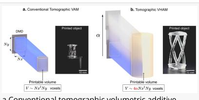
a Conventional tomographic volumetric additive manufacturing. b Tomographic volumetric helical additive manufacturing. Scale bars: 10 mm.
