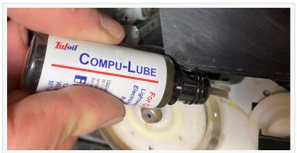
Compu-Lube is a lightweight synthetic oil used to safely lubricate electronics, computers, and high-speed mechanisms such as 3D printers, 3D printer Z screw, computer fans, robotics, printer guide rails, threaded rods, and fine bearings.
