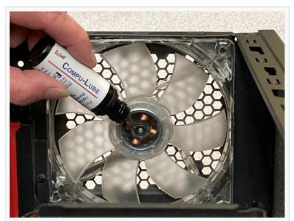
Safely lubricate electronics: Compu-Lube has a high dielectric constant and is safe with computers, electronics, and electromechanical devices.
