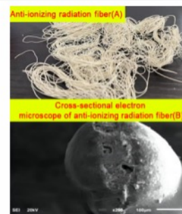
Cross-sectional view of lead-free lightweight ionizing radiation protection fiber
