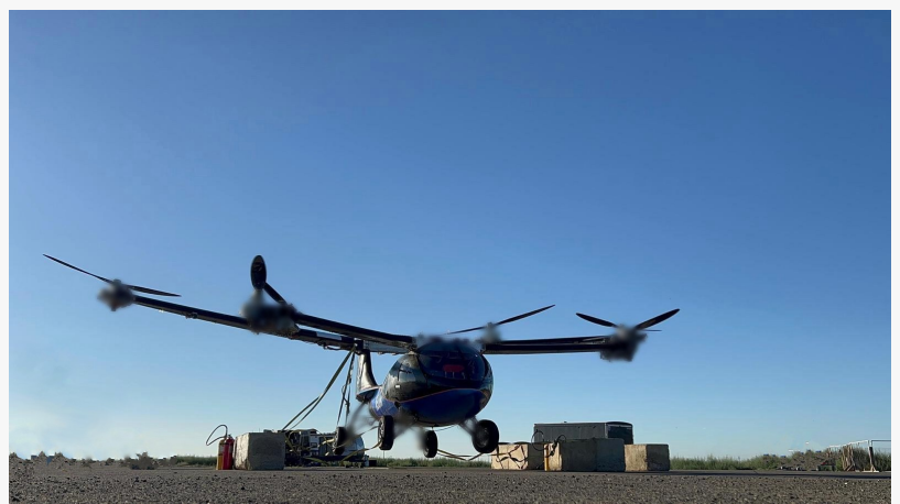
ASKA™ A5 flying car in tethered flight test
