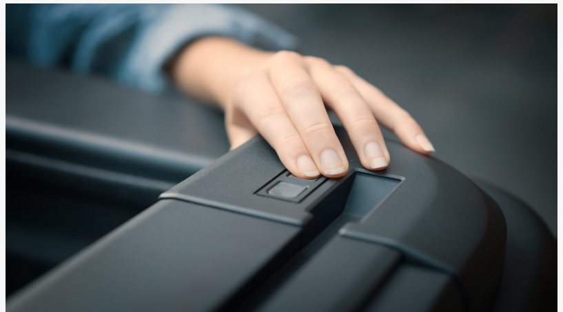
The electric retractable EGR RollTrac bed cover operates with the touch of a button.
