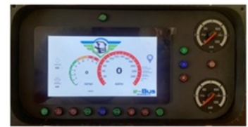
Instrument cluster incorporating telemetry
