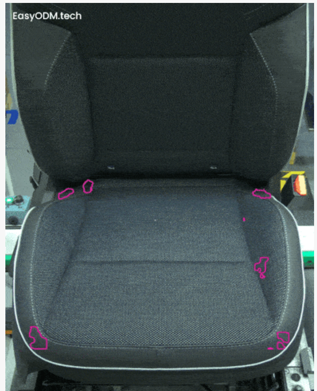
EasyODM software scans segments of the seat for defects, highlighting the affected regions in the image.
