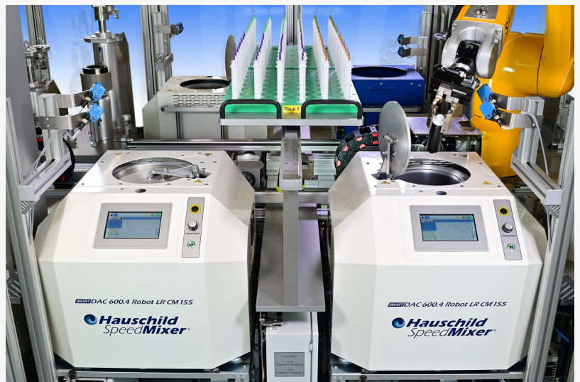
Hauschild SpeedMixer® in a robotic system
