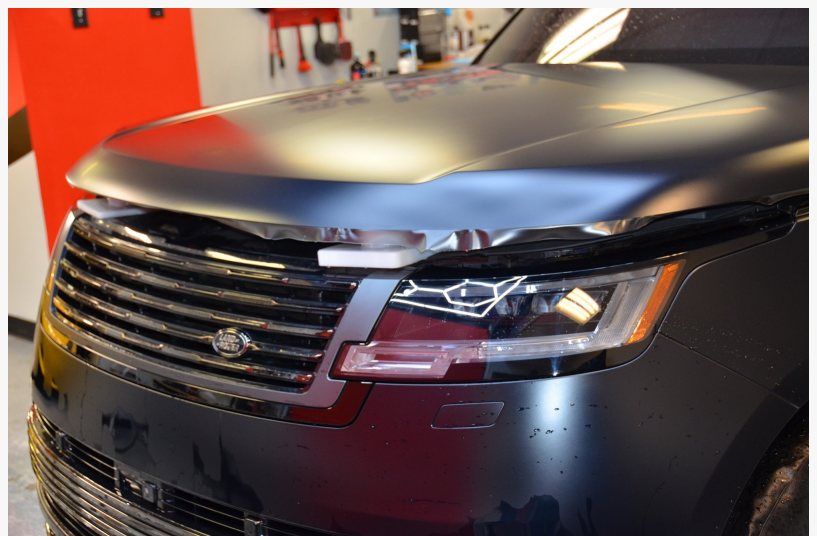
Guardian Matte being installed on a Range Rover
