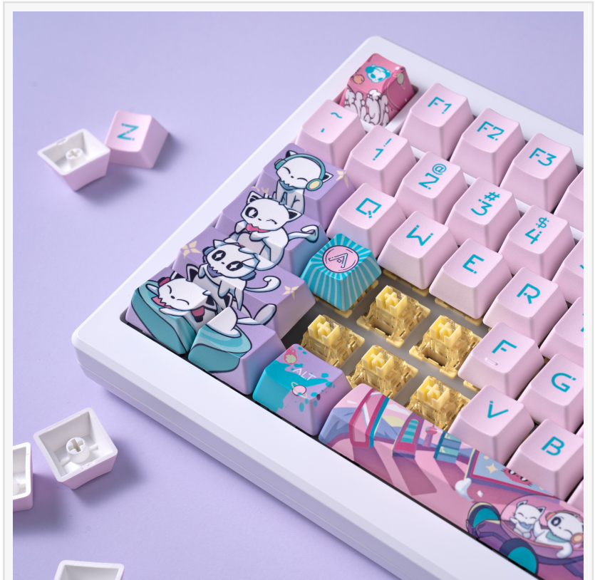
MOD007 PC Keycaps Removed (Showing Magnetic Switches)
