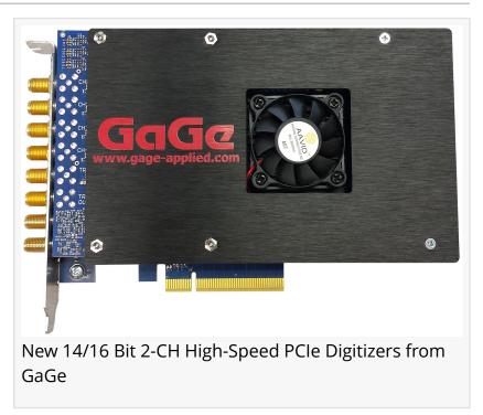
configurations, one with 16-bit and one with 14-bit resolution. For even higher sampling rates, a new <u>14-bit RazorPlus Express</u> option has been added with existing 16-bit model for sampling rates up to 500 MS/s and analog input bandwidth of 250 MHz. GaGe's RazorEdge and RazorPlus Express digitizers boast the industry's best effective number of bits (ENOB) of ~11+ typical.
