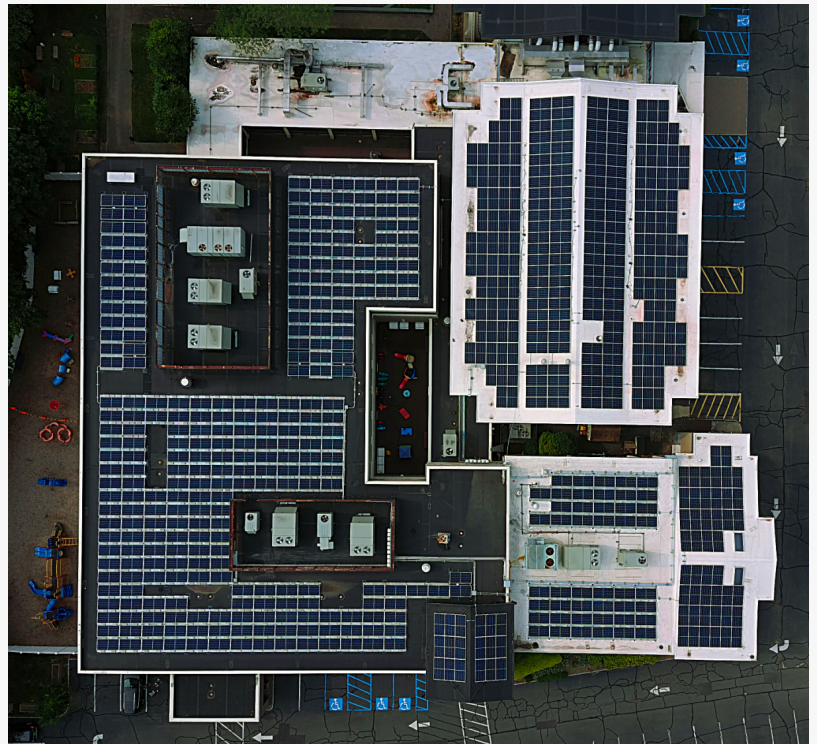
Temple Beth Shalom's 272.7kW Rooftop Solar Arrays
