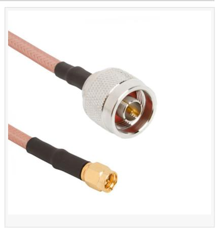
This new cable assembly configuration is designed on RG-142 cable which offers a low loss solution with a bend radius of 1 inch. The N-Type to SMA assembly provides reliable electrical performance up to 11 GHz and features threaded interfaces on both ends for secure mating. Both the N-Type and SMA connectors feature rugged bodies machined from brass. The N-Type connector is nickel-plated while the SMA connector is gold-plated. Both connectors are engineered with gold-plated, brass contacts.
