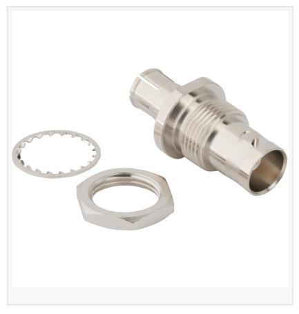
The BNC Jack to BNC push-on plug adapter is manufactured with a nickel-plated, brass body, gold-plated phosphor bronze contact and PTFE insulator. This adapter supports traditional broadcast technology along with newer 4K ultra-HD products which require 12 Gbps data transmission rates. The BNC jack end of the adapter features bayonet coupling for reliable and secure mating while the plug end uses the push-on method.
