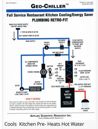
needs, this is made possible with a couple of vales and plumbing retrofit (preset Ratio) flow switch to activate the system. The Hydro turbine unit would have to be made for potable water requirements, and replace the electric motor. The system is energy efficient.
