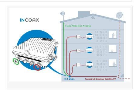
The technology provides operators with shortened deployment times, faster time to revenue of services, and CapEx savings. MoCA Access™ is a technology for fiber or FWA extension that is capable of symmetrical data rates of 2.5 Gbps and up to 3.2 Gbps in some cases over the existing in-building coaxial network.
