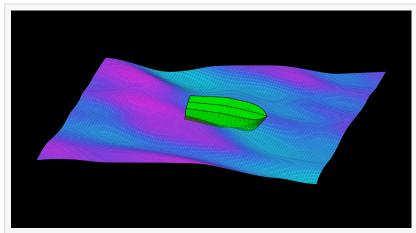
3D hydrodynamic modelling calculates how your individual hull shape will interact with the forecasted wind and wave conditions
