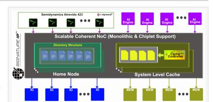
Semidynamics and SignatureIP's provide a fullytested RISC-V, multi-core environment and CHI interconnect for the development of state-of-the-art chip designs
