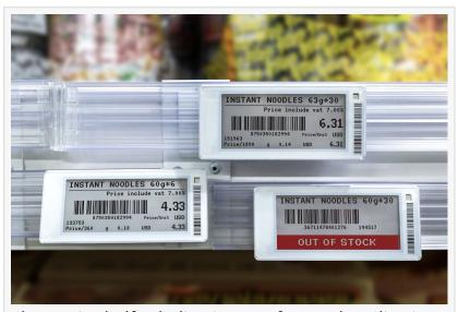
Electronic Shelf Labeling is one of several applications of Bluetooth's new 5.4 PAwR technology that allows multiple devices to advertise and respond with lower energy, more efficiency and more standardized, secure technology.
