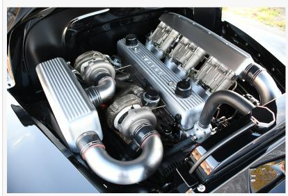
A twin-turbocharged inline-six cylinder engine produces over 500 horsepower.
