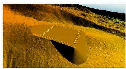
The Create a Flattened Site Plan tool is popular for preplanning the best location, elevation, and required earthworks for the creation of a flat surface in a terrain layer.
