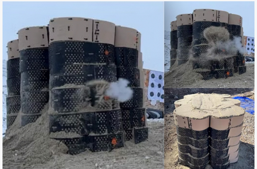
The revetment test wall was subjected to test fire from 50 yard distances and successfully stopped every shot
