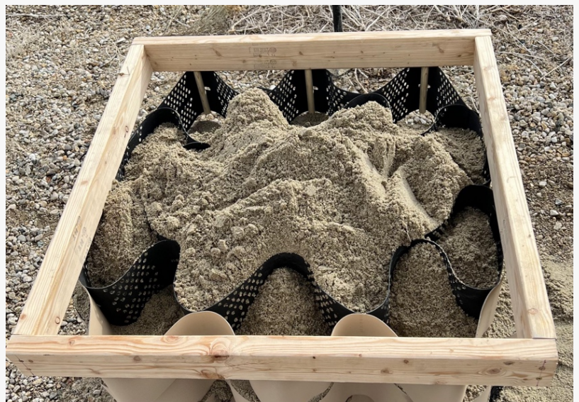
Geocell with material and MICP treatment for creation of "wall blocks"
