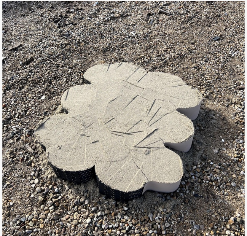
MICP treated soil form created with Geocell is now ready for stacking to create a revetment structures
