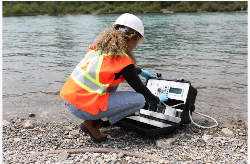
CEC Compact Sampler - sampling at a river bank
