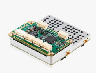
Doodle Labs' Helix Mesh Rider Radio makes use of multi-band and interference-avoidance technology to help drones combat jamming attempts.
