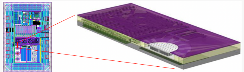
Nanusens pressure sensor with detection circuitry (right) created within the CMOS layers of an ASIC (left)
