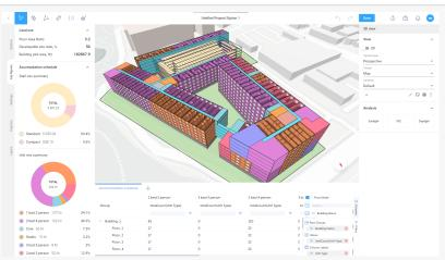
Skema Al's update breaks free of modular design constraints to easily design buildings with geometric variation and non-orthogonal buildings.
