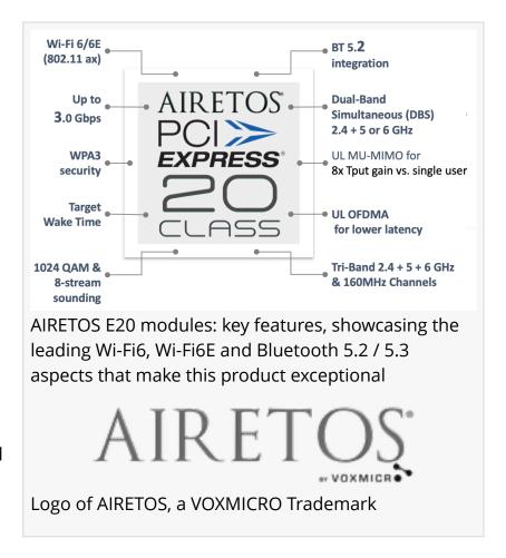
Dual-Band Simultaneous (dual MAC DBS or DBDC, a.k.a. Dual-Band Dual Concurrent) operation for connections up to 3Gbps data rate in a variety of mixed wireless modes (2x2+2x2 11ax).
