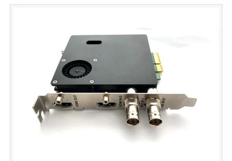
LT-313, 4K Video Capture Card with 2x SDI Inputs and 1x HDMI Input. 1x HDMI Output.
