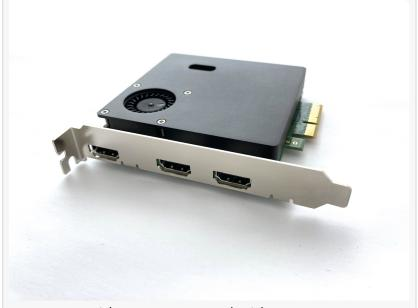
LT-312, 4K Video Capture Card with 2x HDMI Inputs. 1x HDMI Output.
