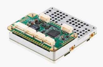
Doodle Labs' Helix Mesh Rider Radio makes use of multi-band and interference-avoidance technology to help drones combat jamming attempts.
