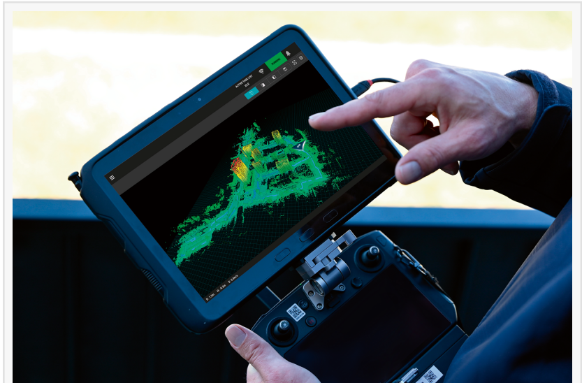
Emesent Commander is a tablet app that makes it easier to plan and control mapping missions.
