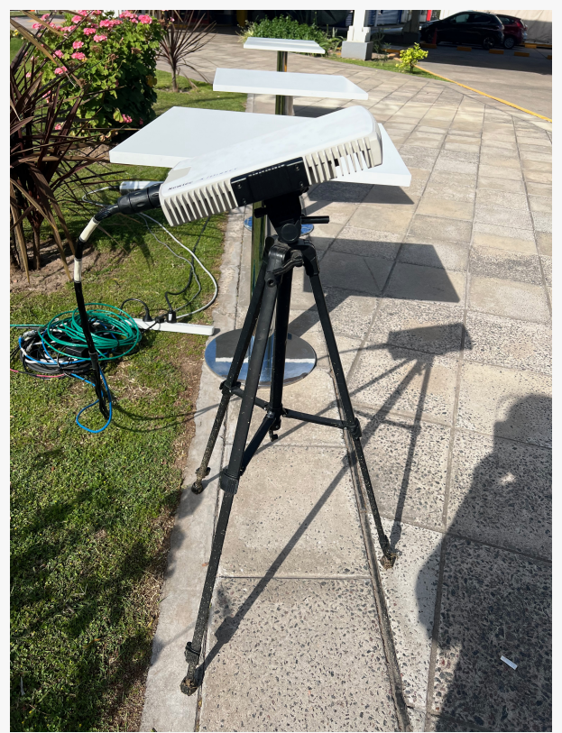
The HiSky terminal integrates the satellite modem and a flat panel antenna
