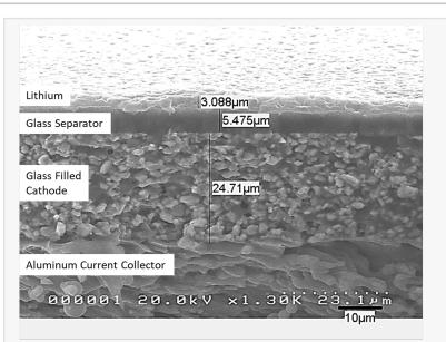
Figure 1: Cross Section of a solid state battery cell consisting of 25 microns of glass electrolyte filled cathode and 5 microns of solid glass separator.
