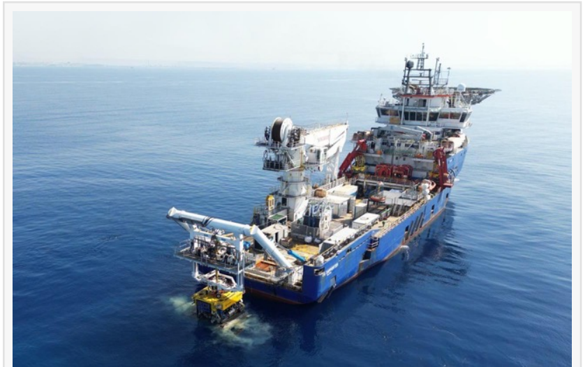
A CSS Subsea ship busy deploying a remote-operated underwater robot (ROV)
