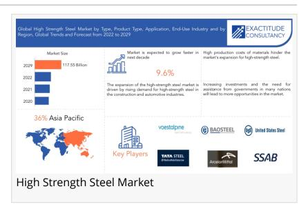
High-strength steels are also known as structural steels because they are commonly used in structural applications. They can be made with or without the addition of a small amount of micro alloying components. Micro alloying elements such as CB, TI, MO, and V are used to create high strength low alloy steels, also known as HSLA steels. Because of the low carbon and alloy
