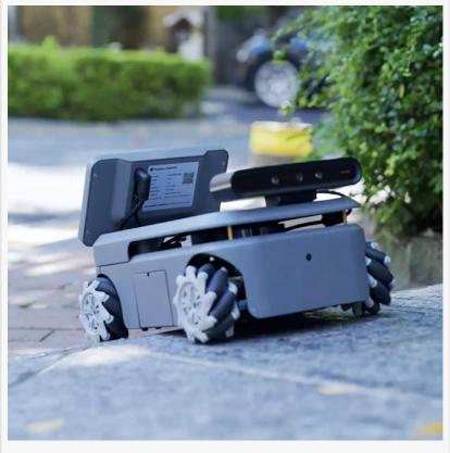
the control and monitoring of the robot's operations. Elephant Robotics also introduces a spare battery option, addressing the demand for extended operational capabilities. With a standby battery life of 328 min and a working battery life of 181 min under full load, the addition of a spare battery effectively doubles myAGV 2023's productivity in long-duration tasks. The optional
